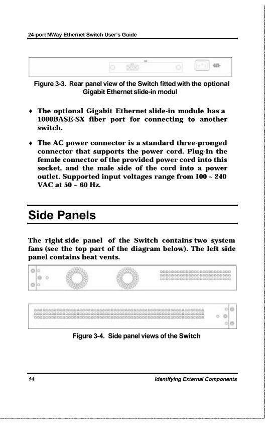
The system fans are used to dissipate heat. The sides of the system also provide heat vents to serve the same purpose. Do not block these openings, and leave at least 6 inches of space at the rear and sides of the switch for proper ventilation. Be reminded that without proper heat dissipation and air circulation, system components might overheat, which could lead to system failure.
